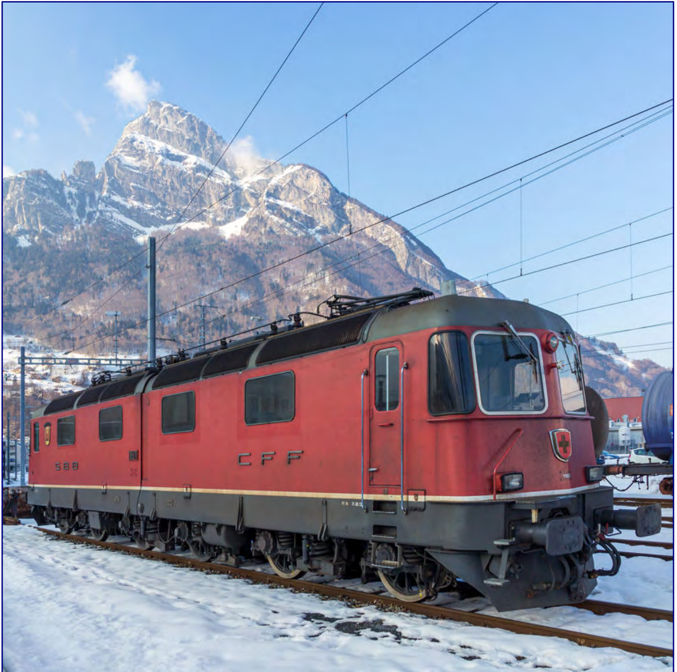
The same locomotive as on page 5 is shown here after its modernisation on 17 February 2013 in Buchs/SG. The split locomotive body, which only the two prototypes had, is clearly visible. Photo: Joachim Kohler (CC-BY-SA-4.0)
