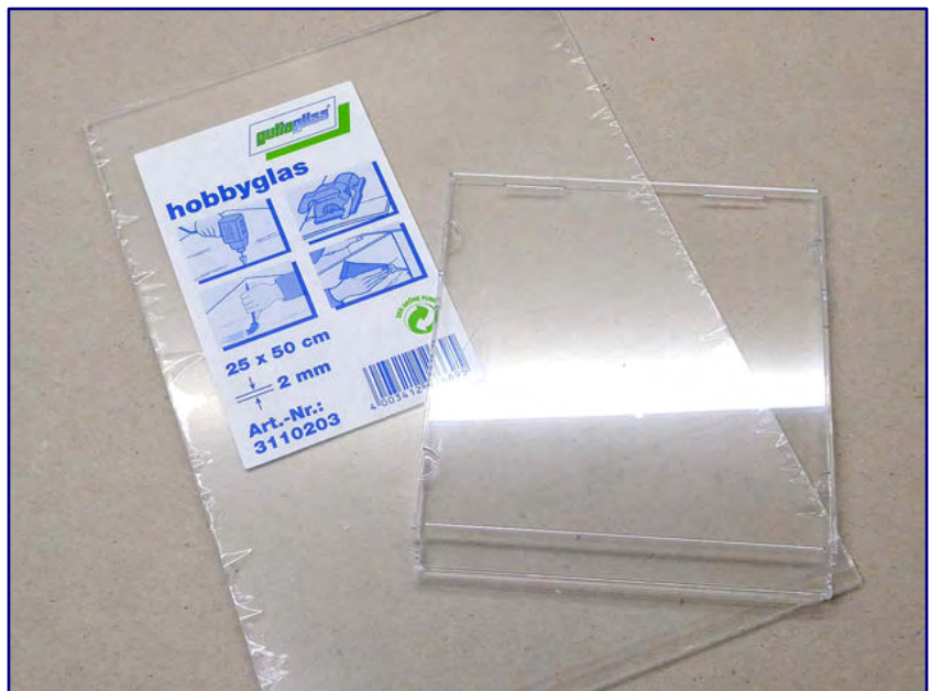
Our material of choice is crystal-clear polystyrene. Alternatively, CD sleeves can also be processed.
