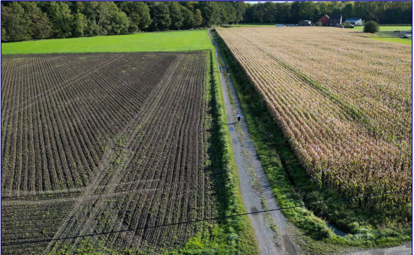
The layout of a paved path with rain (left) and drainage ditch (right) can be seen here just as well as the many places where greenery penetrates even the compacted subsoil with a gravel layer.
