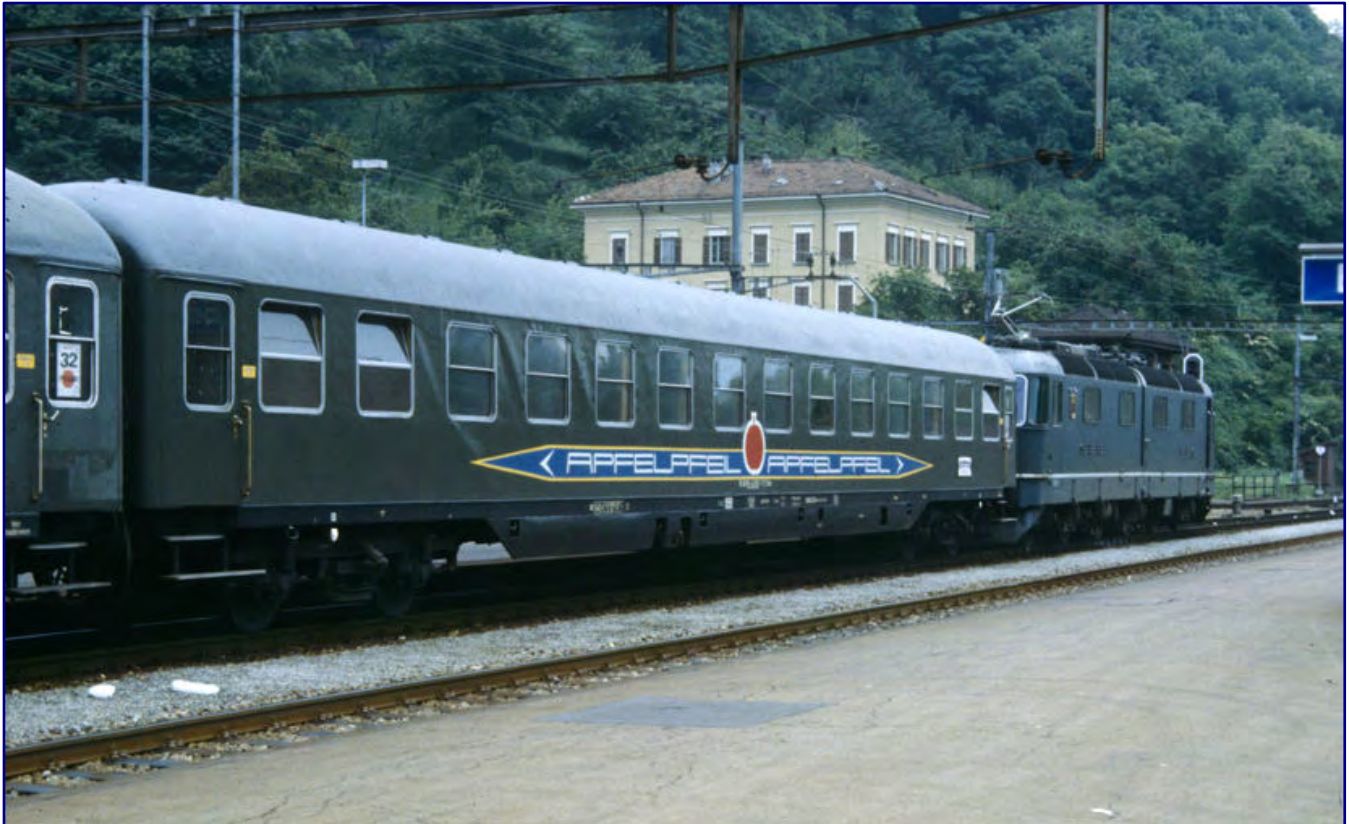
Re 6/6 11601 "Wolhusen" was the first of two prototypes for the new Gotthard locomotive. It can be seen here with wagons from the Apfelpfeil organisation between 1973 and 1980. Photo: ETH Library Zurich, Image Archive (Photographer: Hans-Peter Bärtschi / SIK_03-107655 / CC BY-SA 4.0)
