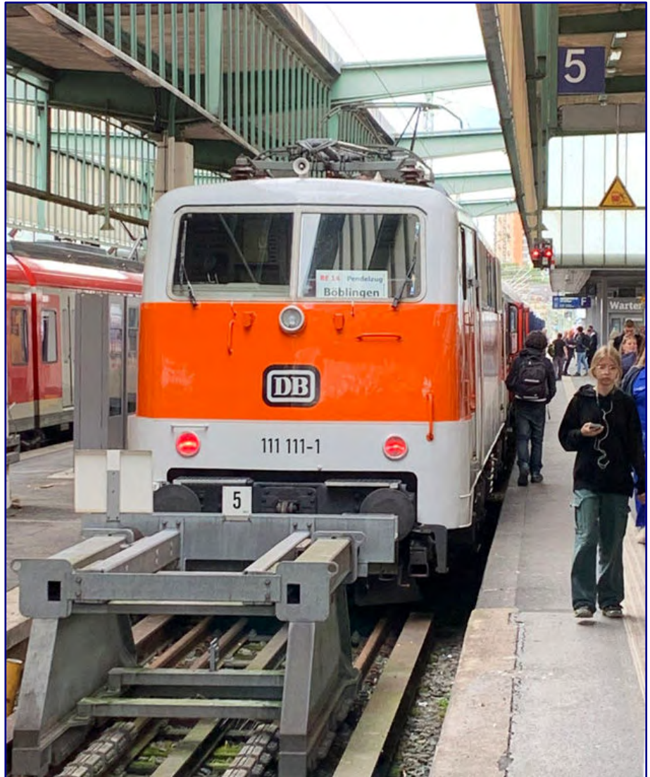
If we look at 111 111-1 during its turnaround at Stuttgart main station on 7 August 2023, we hardly notice the thin contact wire above it. But, the single-arm pantograph also gives a significantly different impression than the Märklin conversions. Photo: Alexander Hock
